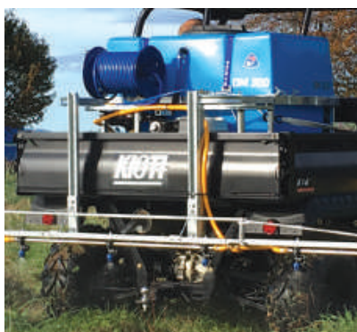
OPTIONAL SMART-FIT BOOMS, ALLOWING TAILGATE TO REMAIN CLOSED
