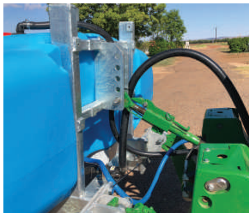
OPTIONAL ADAPTOR FRONT MOUNT 3 POINT LINKAGE
